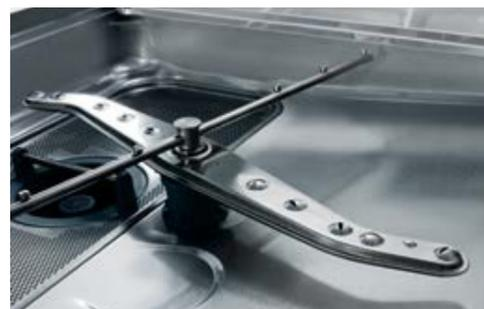
**Seamless wash tank.** The absence of dirt traps in the Advantage's wash tank means that debris, dirt and grease are effortlessly expelled. Because the tank is fabricated from a single sheet of metal with seamless, rounded corners, and because the tank's floor is inclined, all debris collects in the dirty wash water which is automatically drawn towards the filter and drain pump.
